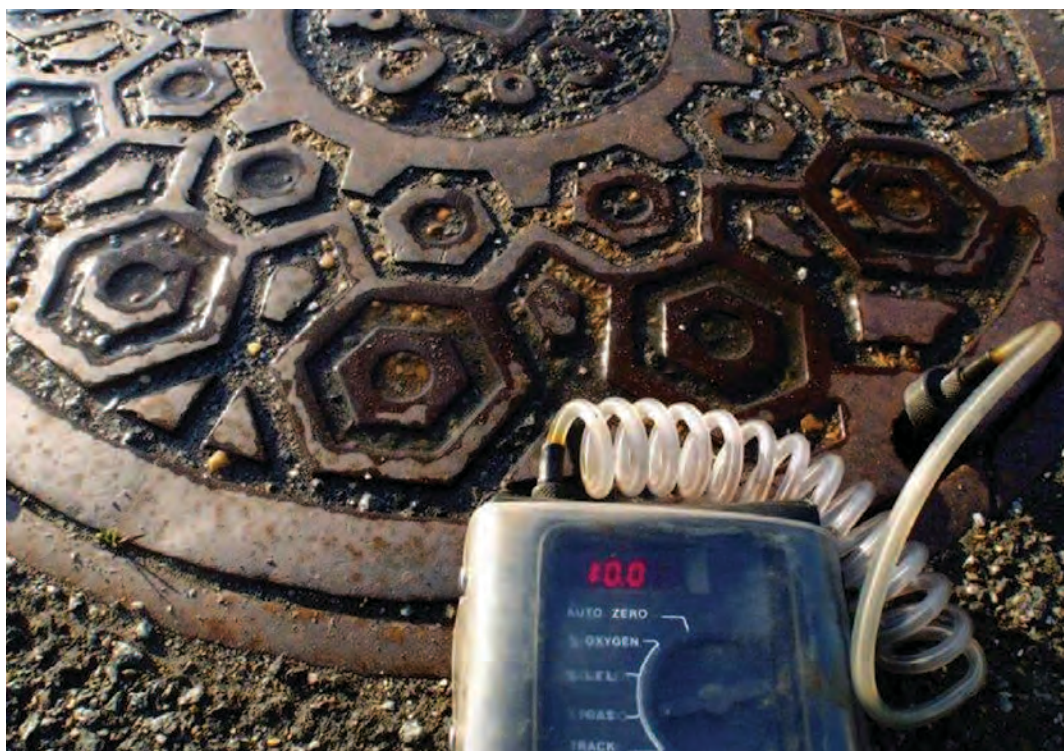
ABOVE: An accident waiting to happen: Methane at 10% (100,000 ppm) gas concentration —well above the lower explosive limit of 5% —was measured in a telecommunications manhole in Washington, D.C. Driving every street in the District, researchers found 5,893 natural gas leaks from the city’s aging pipe system. Photo: Robert B. Jackson, Duke University. BELOW: Concentrations of methane from leaks measured in Boston. Graphic: Robert B. Jackson, Duke University
